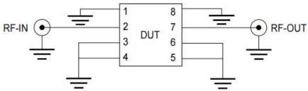
Fig 1. Block Diagram of Test Circuit used for characterization. Die is packaged in 2x2mm, 8-lead MCLP and soldered on testboard TB-1041-5-63+
