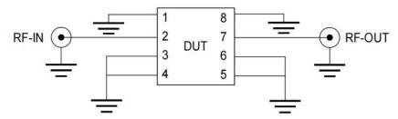
Fig 1. Block Diagram of Test Circuit used for characterization. Die is packaged in 2x2mm, 8-lead MCLP and soldered on testboard TB-1041-8-63+
